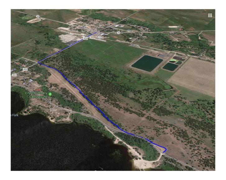
The pathway concept is an 6 to 8 foot pathway, with a 5 foot (minimum 3 foot) break between the path and roadway. The pathway surface may consist of  $\frac{3}{4}$  inch or less gravel and/or possibly Crusher Stone material.
